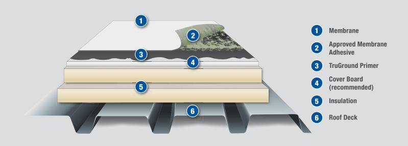
If an FM rated roof assembly including electronic leak detection is required, one of the above listed assemblies must be used. In cases where the building is not FM insured, but a Carlisle Total System warranty is desired, the assemblies listed above or below may be used:
