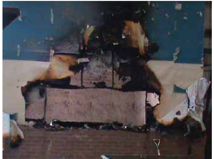
Fire-Resist Barritech VP over R2+ SHEATHE Insulation Window head condition over NFPA 285 Test
